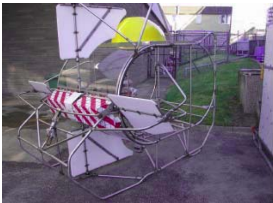
ROV to take samples of sediment under tow
